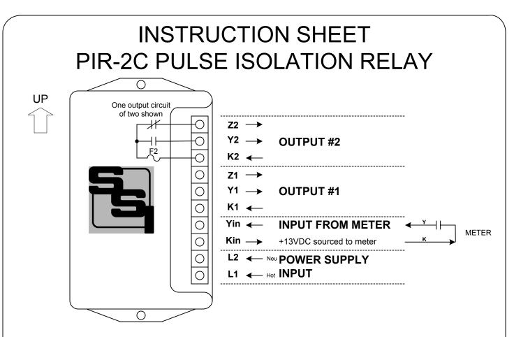
**MOUNTING POSITION -** Because the PIR-2C contains mercury-wetted relays, it must be mounted in a vertical position to operate correctly.
