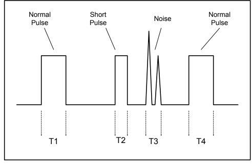
by measuring the time the input voltage is present. If the input voltage is present for less than 20 to 25 milliseconds. it is assumed to be noise. An input of longer duration is classified as a valid input and an output will occur. In the illustration to the left, the normal pulses with time durations of T1 and T4 will cause an output. The short pulse of time duration
